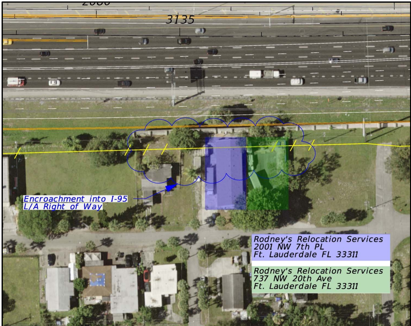
Figure 29 | Right-of-Way Encroachments along East Side of SR9/I-95
