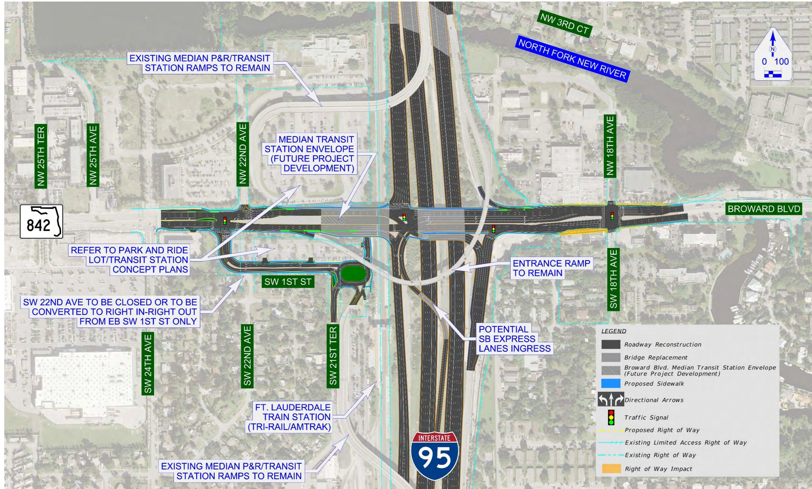
Figure E-6 | Preferred Alternative (Alternative 2B – Modified Displaced Left with Combined Roundabout)
